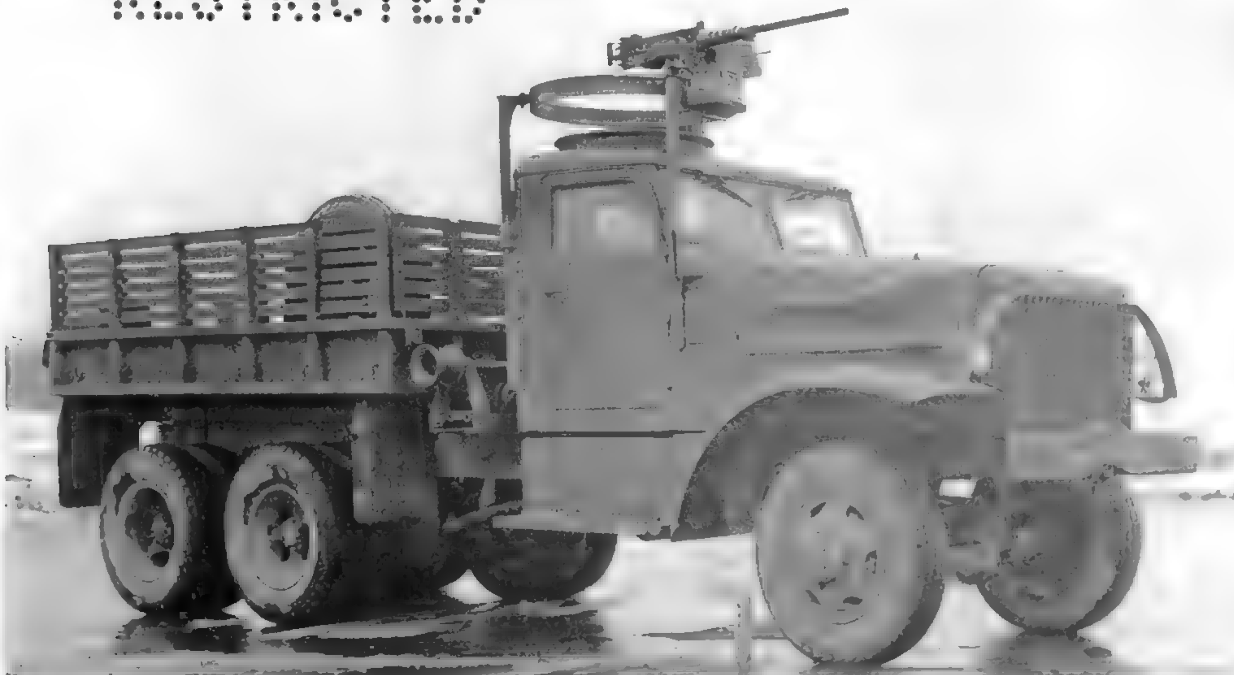
This early Corbitt 6-ton has had an anti-aircraft machine-gun mount added above its enclosed cab. This vehicle also has a steel cargo bed — a feature discontinued in 1942. The midship winch is visible between the cab and bed. (National Archives and Records Administration photo)
